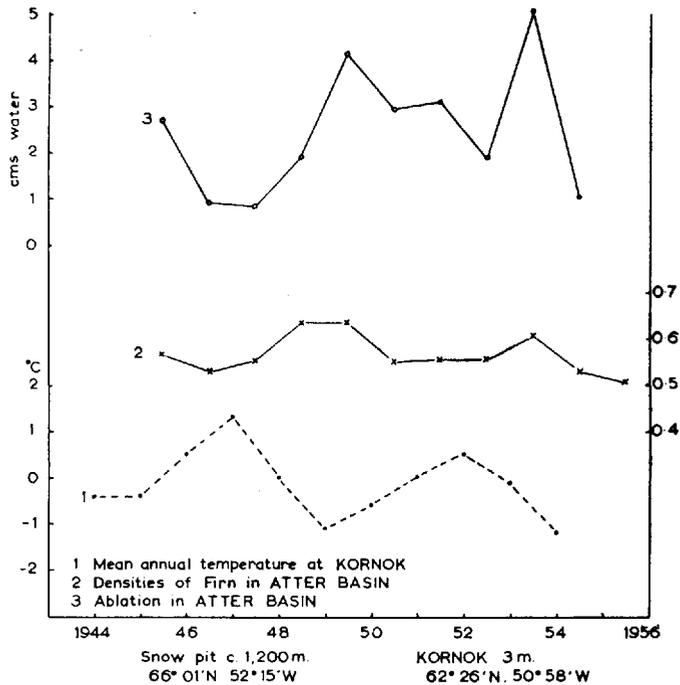
Fig. 3. Ablation and densities of firn in Atter Basin compared with the mean annual temperature at Kornok
