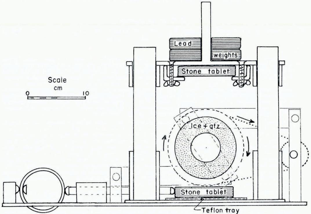
Fig. 1. Longitudinal section of equipment for simulated glacial abrasion.
