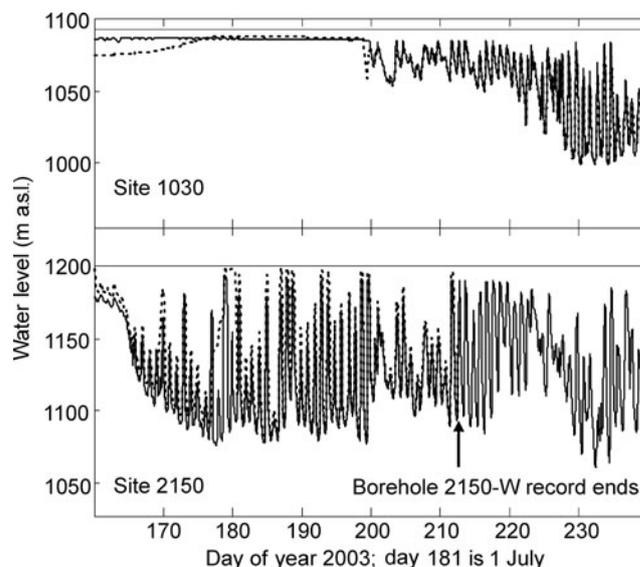
**Fig. 5.** Borehole water-level records from two sites in the ablation area in 2003. Eastern boreholes (E) are solid lines and western boreholes (W) are dashed lines. Horizontal line is the glacier surface. Records can be difficult to distinguish from each other because water levels match closely.
