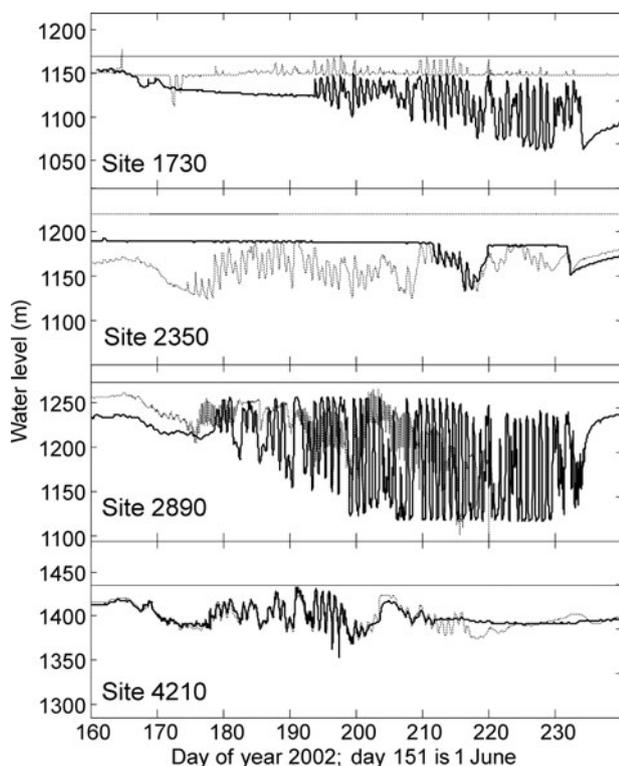
**Fig. 4.** Borehole water-level records from four sites in the ablation area in 2002. Eastern boreholes (E) are solid lines, and western boreholes (W) are dashed lines. Horizontal line is the glacier surface. The records of sites 2350 and 4210 can be difficult to distinguish from each other because the water levels match closely.
