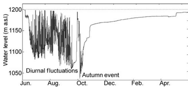
**Fig. 2.** Year-long water-level record from borehole 2150-E beginning in June 2003 when the borehole was drilled. Straight line is the glacier surface. The large diurnal water-level fluctuations of summer and the high stable pressure of winter are shown. The autumn event is common to many boreholes after diurnal fluctuations in water level have ended, and is discussed more by Fudge and others (2005).
