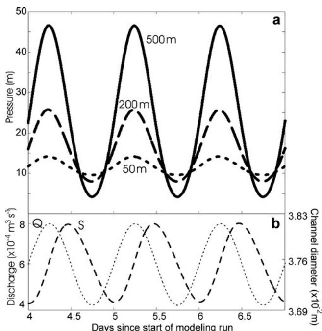
**Fig. 12.** (a) Modeled water-level fluctuations with different connecting pipe lengths. (b) Discharge ( $Q$ ) and pipe diameter ( $S$ ).
