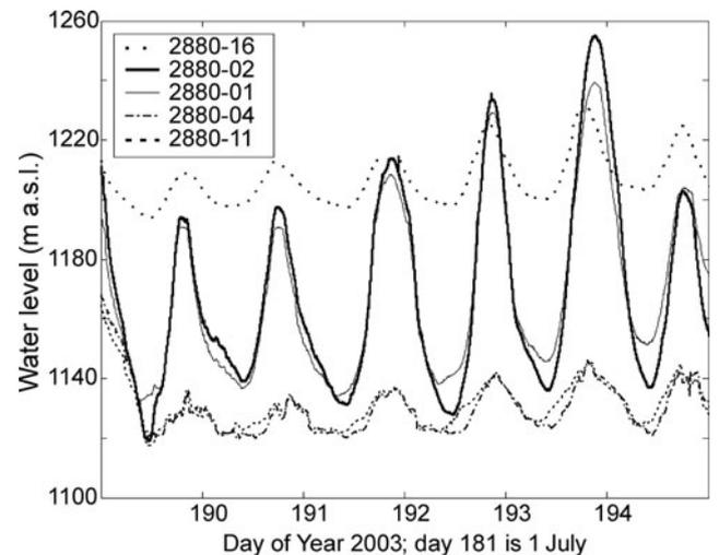
**Fig. 9.** Diurnal water-level fluctuations in five boreholes illustrate the three distinct types observed at site 2880 (the 16-borehole grid). Boreholes 01 and 02 are in cluster 1 (solid lines), boreholes 04 and 11 are in cluster 2 (dashed lines), and borehole 16 is not clustered with other boreholes with diurnal fluctuations (dotted line).
