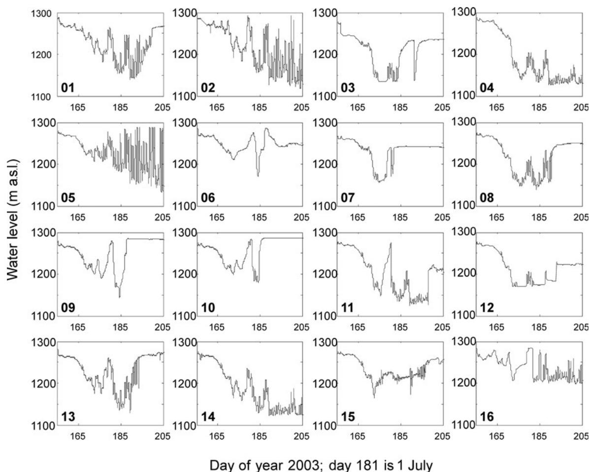
**Fig. 6.** Borehole water-level records from the 16 boreholes at site 2880, oriented looking up-glacier with boreholes 1–4 highest on the glacier and boreholes 1, 5, 9 and 13 on the east. Glacier surface is at 1285 m a.s.l.
