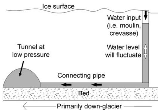
**Fig. 11.** Schematic of model set-up for numerical test. The water level will fluctuate in the moulin based on the pressure in the pipe and serves as a proxy for the water level in a connected borehole.
