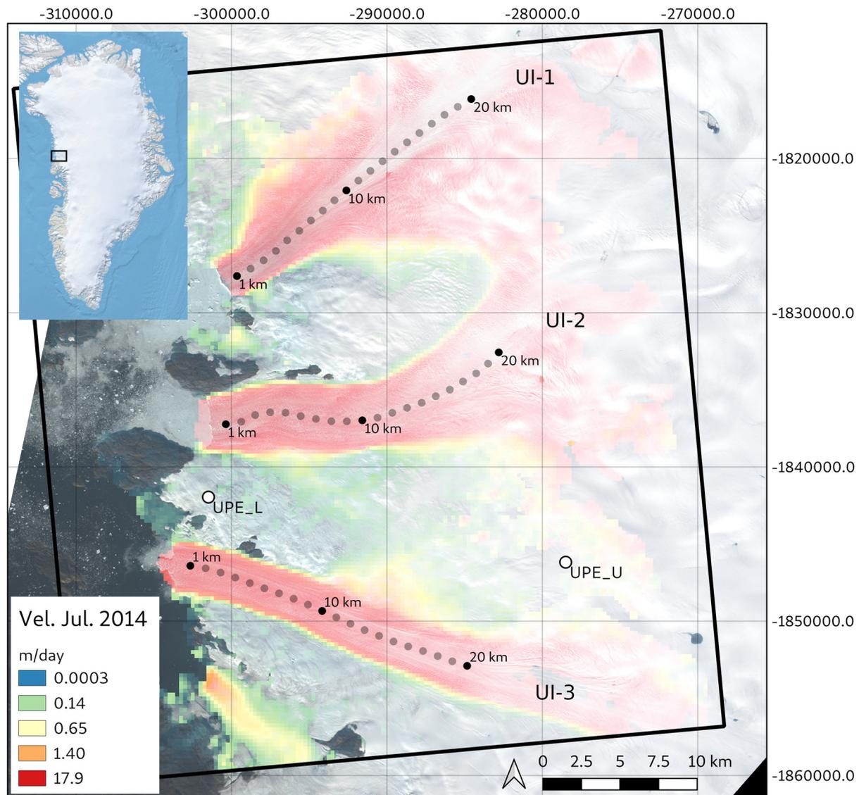
**Fig. 1.** Upernavik Isstrøm area seen from Landsat 8 (28/08/2014). Overlaid is a COSMO-SkyMed-derived velocity map from 23/07/2014. Black dots indicate data sampling points in km from the 2014 front corresponding to the locations presented in Figures 4–6. The three main outlet glaciers are designated UI-1, UI-2 and UI-3. Circles indicate the location of PROMICE weather stations. The black box outlines the COSMO-SkyMed coverage. Projected coordinate system EPSG:3413.
