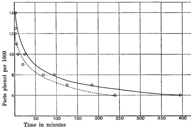
Fig. 12. Effect of varying the concentration of phenol upon the time taken for disinfection of (a) *B. paratyphosus*, dotted curve (Exp. 21. 6. 06, Table XVI): (b) *Staph. aureus*, continuous curve (Table XVII).
