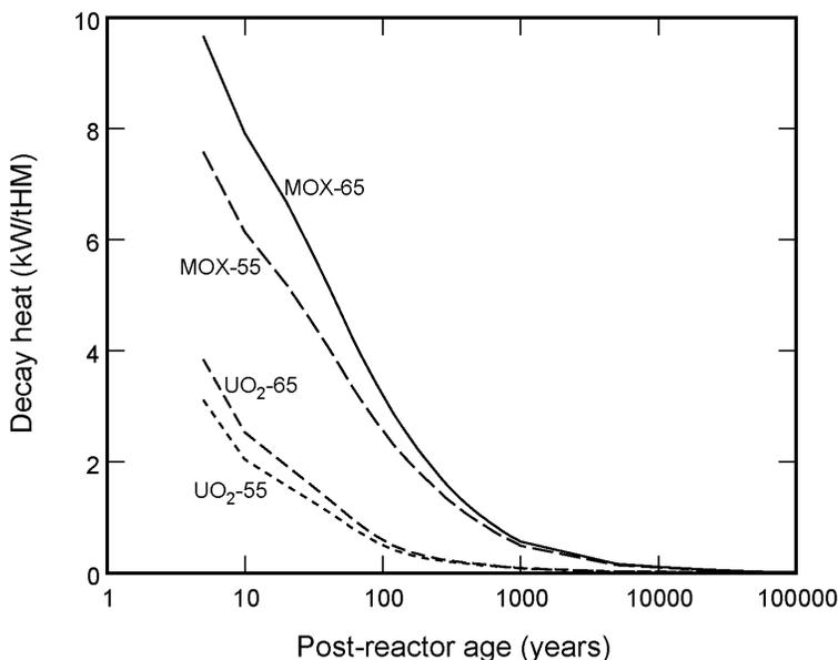
FIG. 3. Decay heat outputs for the four fuel type/burn up combinations used in the modelling.
