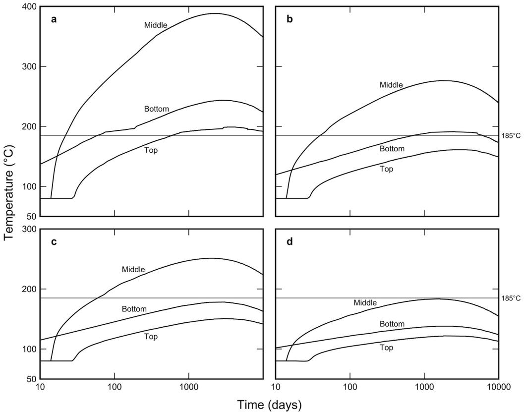
FIG. 9. Evolution of temperatures at the outer surfaces of the containers in batches of 5 emplaced at 7 day intervals: (a) 600 pins of 40 year old MOX-55; (b) 250 pins of 20 year old MOX-65; (c) 250 pins of 30 year old MOX-65; and (d) 600 pins of 30 year old UO<sub>2</sub>-65. Top, middle and bottom refer to the level in the stack.
