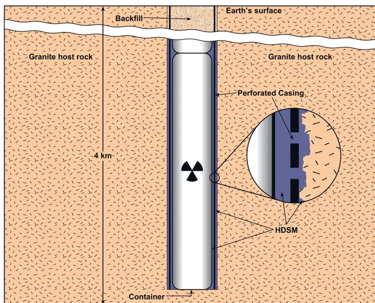
FIG. 2. Deep borehole disposal concept LTVDD-2a with inset showing detail of the high-density support matrix (HDSM) (not to scale).
