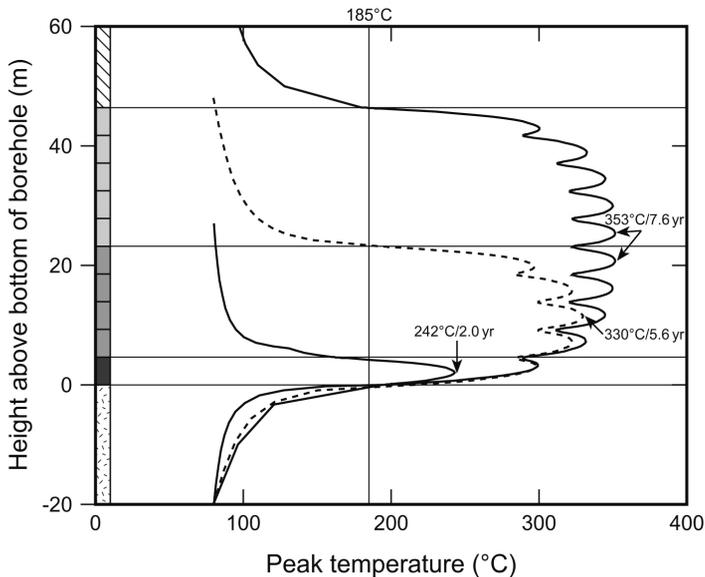
FIG. 7. Comparison of peak temperatures on the outer surface of the stack for 1, 5 and 10 containers with 350 pins of 30 year old MOX-65 emplaced at 7 day intervals.
