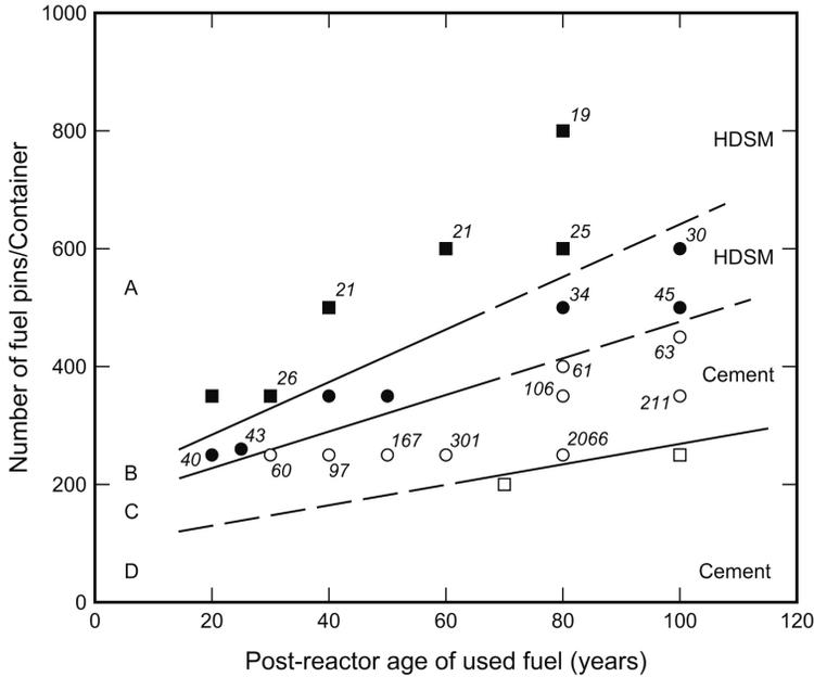
FIG. 10. Outcomes (see text) of temperature modelling for DBD of 5-container batches of MOX-65 as a function of age of the fuel and number of pins per container. Symbols indicate outcome; adjacent numbers indicate time in days to first melting of the HDSM (if used).
