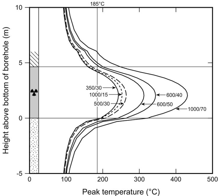
FIG. 4. Examples of peak temperatures at the outer surfaces of single containers. The short dashed line is for  $\text{UO}_2\text{-65}$ , the long dashed line for  $\text{MOX-55}$  and the solid lines for  $\text{MOX-65}$ ; arrows indicate the number of pins per container and the age of the fuel (years).
