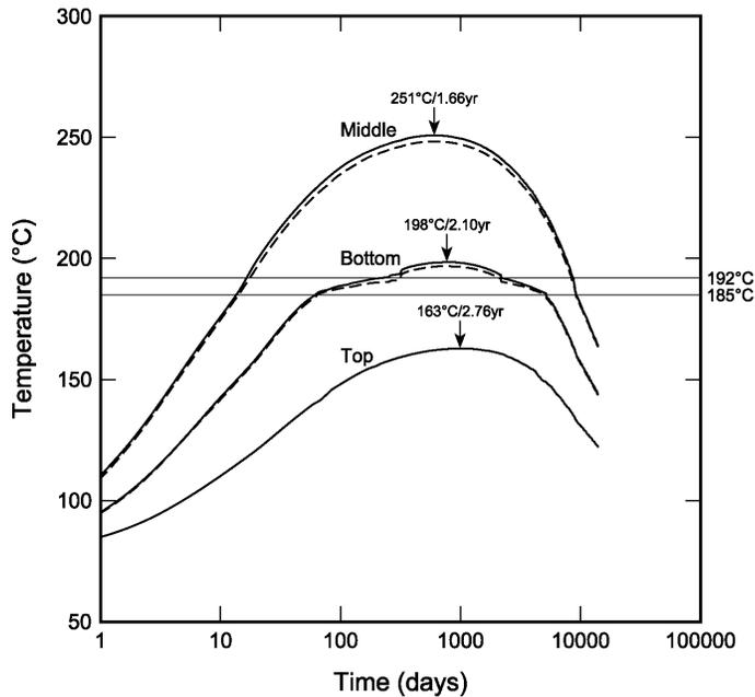
FIG. 6. Evolution of temperatures for a single container with 1000 pins of 15 year old  $UO_2-65$ . Solid lines are for points on the outer surface of the container and dashed lines for points on the borehole wall at the top, middle and bottom of the container. Arrows indicate peak temperatures and the times at which they are reached.
