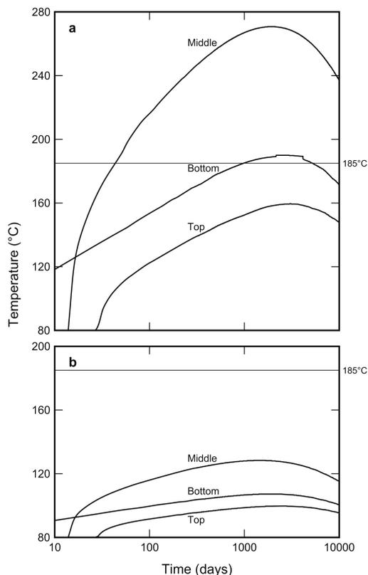
FIG. 11. Evolution of temperature at the outer surfaces of the containers in batches of 5 emplaced at 7 day intervals: (a) 260 pins of 25 year old MOX-65; and (b) 260 pins of 25 year old UO<sub>2</sub>-65.
