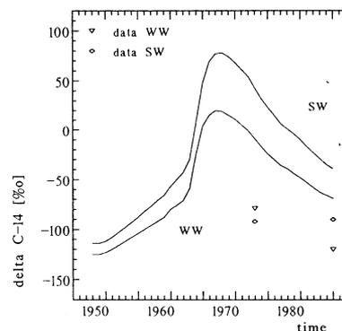
Fig 3B. Calculated  $^{14}\text{C}$  concentration of SW and WW as a function of time. The time constant for carbon exchange of the SW is set to 4 yr and the entrainment rate of WDW into the winter mixed layer to  $33\text{m yr}^{-1}$ .
