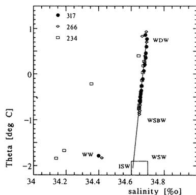
Fig 7A. Potential temperature vs salinity plots – ANT V stations. The mixing line between WDW and WSBW is extrapolated to a temperature of  $-2.05^{\circ}\text{C}$ . WSW marks the  $\theta/S$  characteristic of WSW. The  $\theta/S$  characteristic of ISW is indicated.
