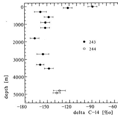
Fig 2B. AMS  $^{14}\text{C}$  profile from ANT III station 243 (lower two data points taken from station 244 to extend the profile into WSBW). Samples were measured at the Zürich AMS facility and taken from Schlosser *et al* (1987).
