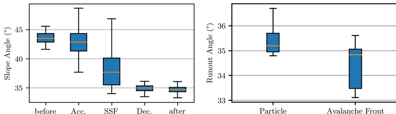
**Figure 9.** The box plot illustrates the slope angles for all measurements corresponding to the identified dynamic states. It also includes the run-out angles for the AvaNodes, as well as the documented avalanche fronts.
