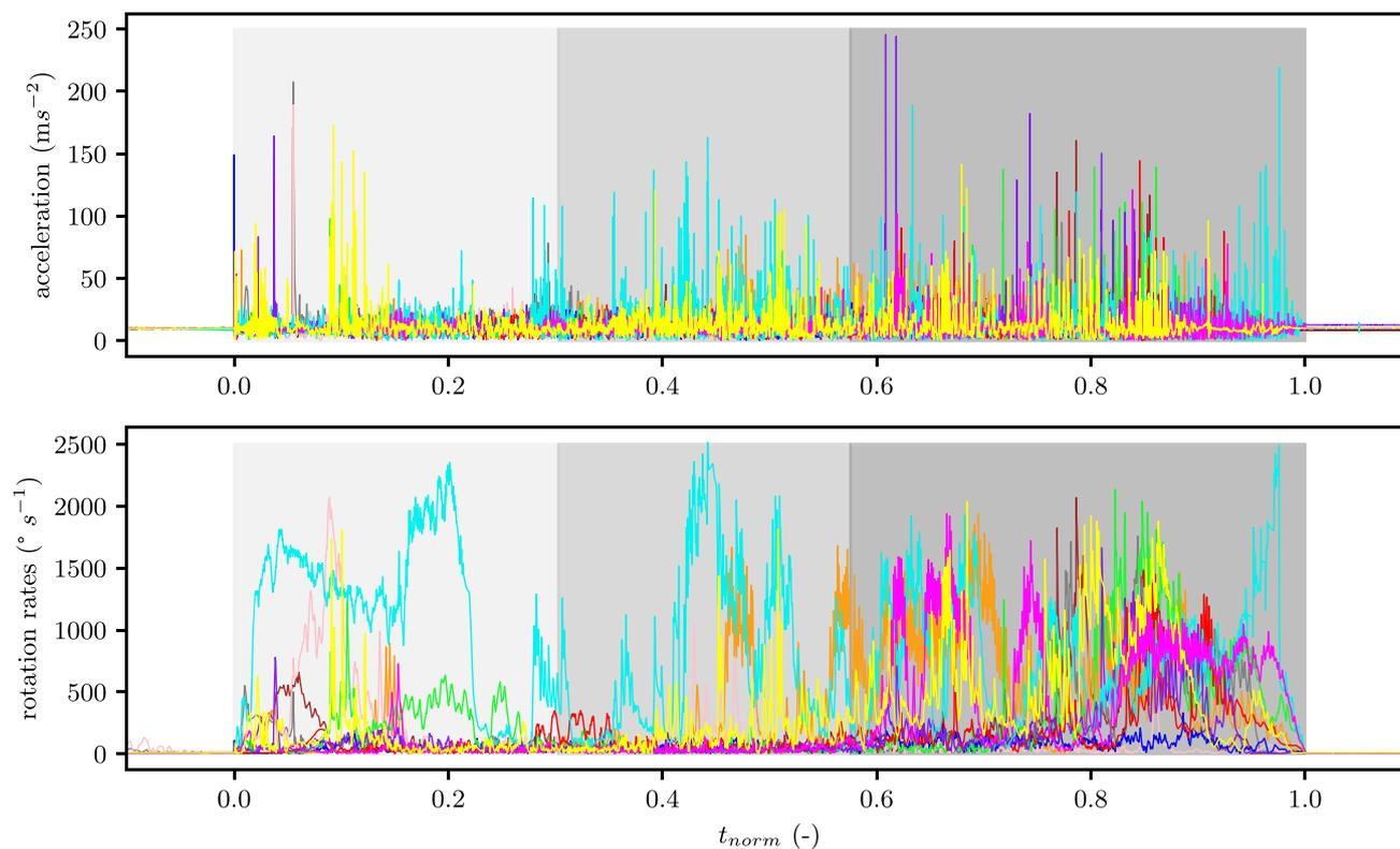
**Figure 6.** IMU absolute acceleration in the top panel and IMU rotation rates in the bottom panel with normalised times. Acceleration state in light grey, flow state in grey and deceleration state in dark grey. The AvaNodes with higher density are shown in green (C07-220222), cyan (C06-230203) and magenta (C07-230204).
