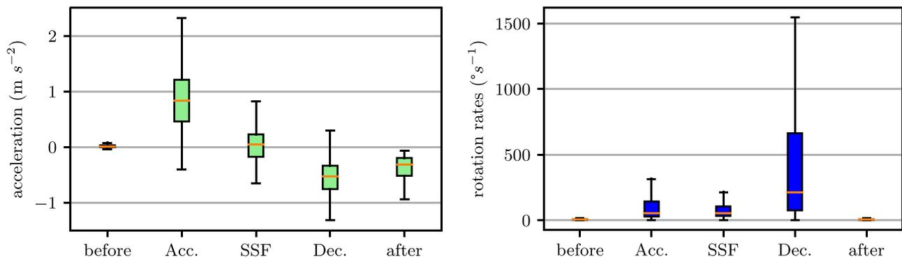
**Figure 8.** This Figure shows the GNSS Doppler accelerations  $a_d$  and rotation rates measured with IMU. All panels are divided into three flow states, including before and after movement indication.
