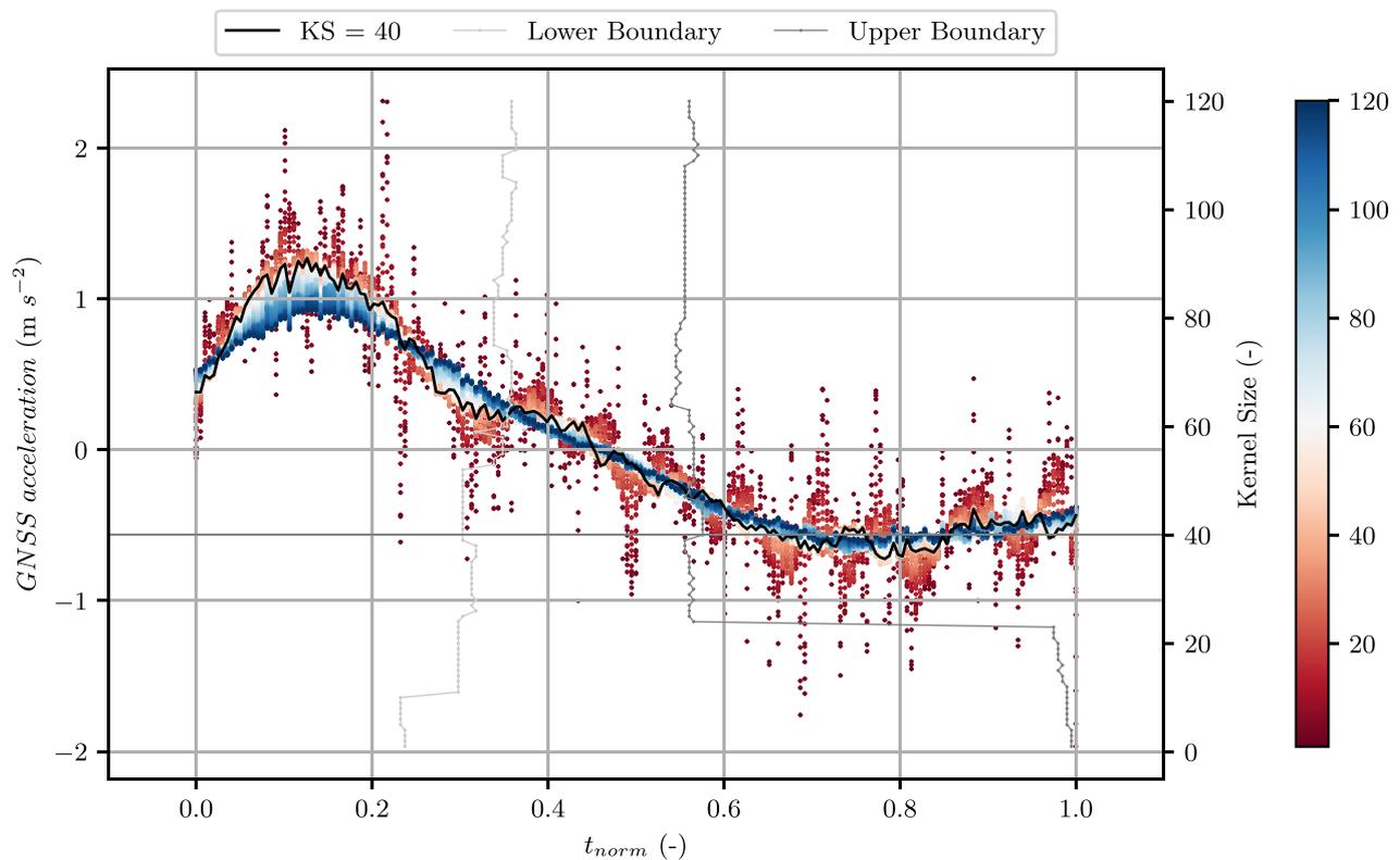
**Figure 11.** This figure shows the evolution of the mean GNSS accelerations when varying the kernel size between 1 and 120 (red to blue dots). Since for the flow state analysis, kernel size = 40 is used, this is plotted as a black line. The light grey and grey line indicate the boundaries between the flow states for different kernel sizes.
