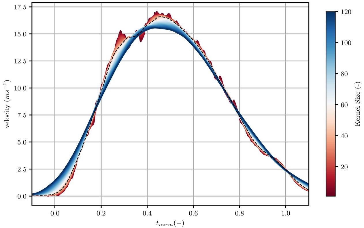
**Figure 12.** This figure shows the velocity distribution of AvaNode C10 at experiment 220222, smoothed with different kernel sizes. The black dashed line indicates the smoothed velocity distribution at kernel size 40, while the distribution from kernel size 1 to 120 is displayed with the colours from red to blue.
