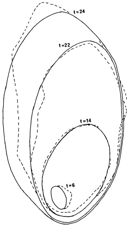
Fig. 10. Fire 53: The observed (dotted) and predicted positions of the fire front at 6, 14, 22 and 24 minutes.
