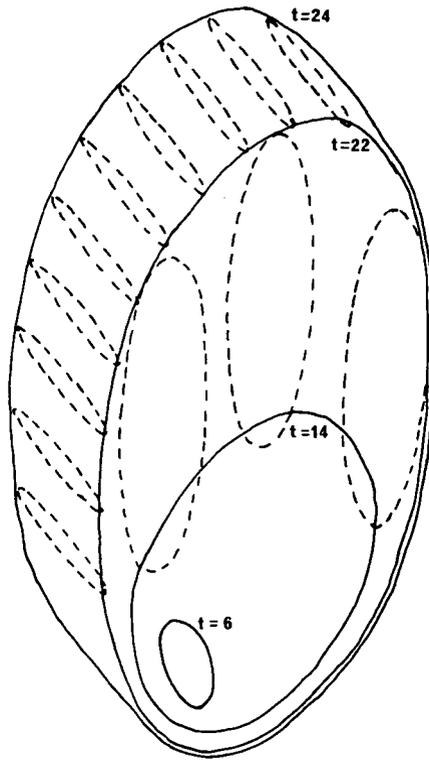
Fig. 9. Fire 53: The predicted fire fronts at 6, 14, 22 and 24 minutes, and the Huygens' ellipses (dotted) used to step from  $t = 14$  to  $t = 22$  ( $\beta = -22^\circ$ ,  $af = 4.2$ ,  $ag = 3.8$ ,  $ah = 1.1$ ) and from  $t = 22$  to  $t = 24$  ( $\beta = 20^\circ$ ,  $af = 1.9$ ,  $ag = 1.8$ ,  $ah = 0.2$ ).
