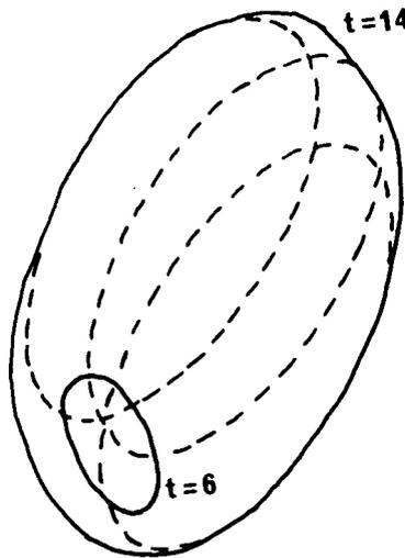
Fig. 8. Fire 53: The predicted (elliptical) fire front at 6 minutes ( $\beta = 0^\circ$ ,  $af = 1.2$ ,  $ag = 0.8$ ,  $ah = 0.6$ ); the Huygens' ellipses (shown dotted) used to step from  $t = 6$  to  $t = 14$  ( $\beta = -55^\circ$ ,  $af = 3.5$ ,  $ag = 3.1$ ,  $ah = 1.7$ ); and the resulting predicted fire front at 14 minutes.
