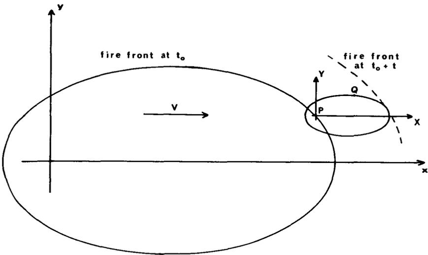
Fig. 5. Huygens' principle for a steady wind  $V$ .
