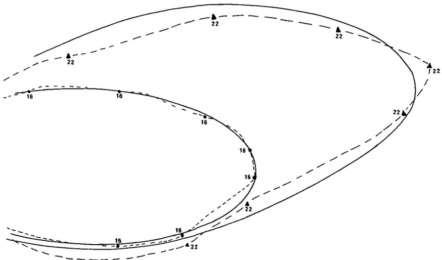
Fig. 7. Fire 7: the fitted fire front at 16 minutes and the predicted fire front at 22 minutes after a single change of wind through  $30^\circ$  at 16 minutes. The observed fire fronts are shown dotted.
