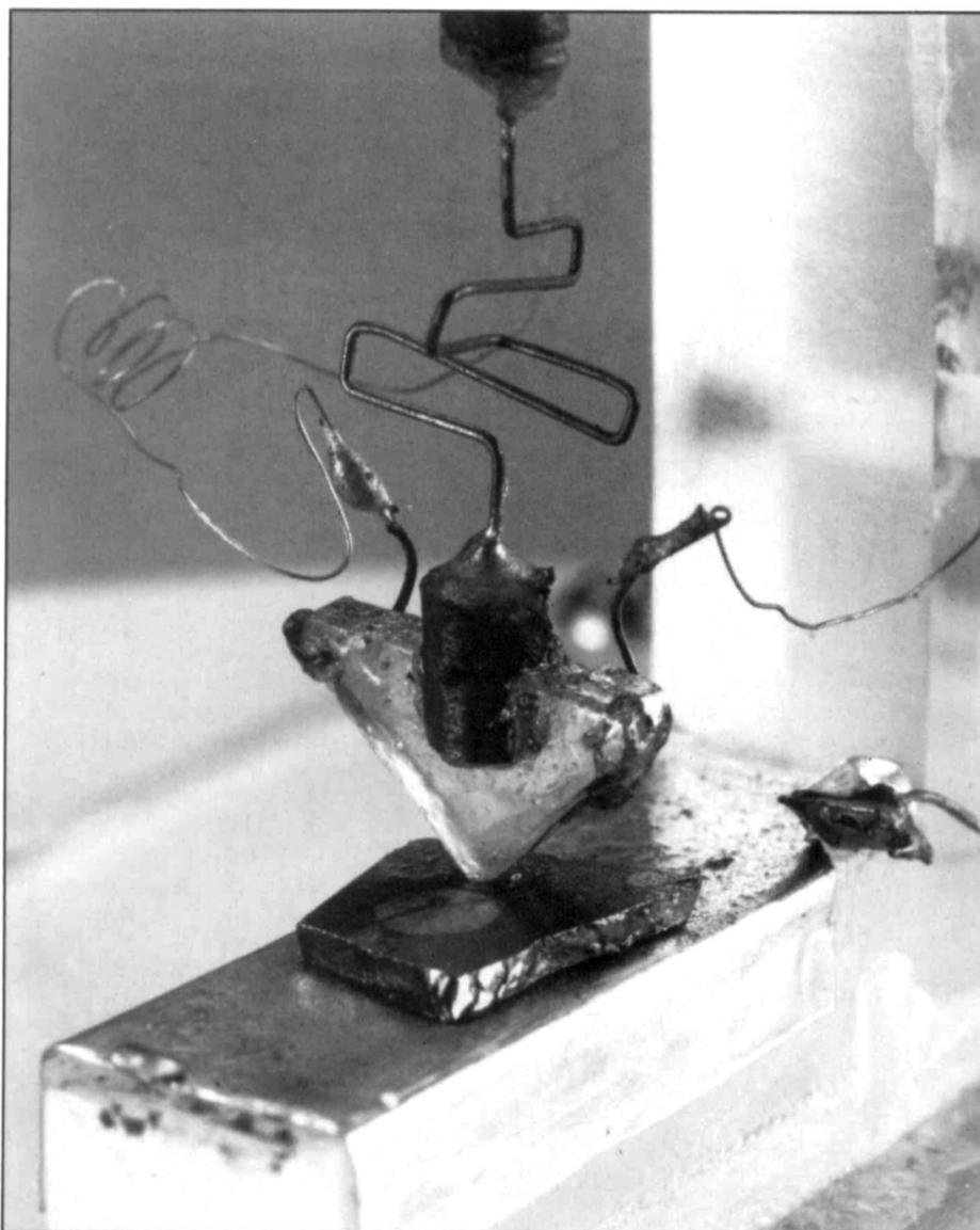
*The first transistors assembled by their inventors at Bell Laboratories were primitive by today's standards. This first transistor, a "point-contact" type, amplified electrical signals by passing them through a solid semiconductor material, basically the same operation performed by present "junction" transistors. Photo courtesy of AT&T Archives.*
