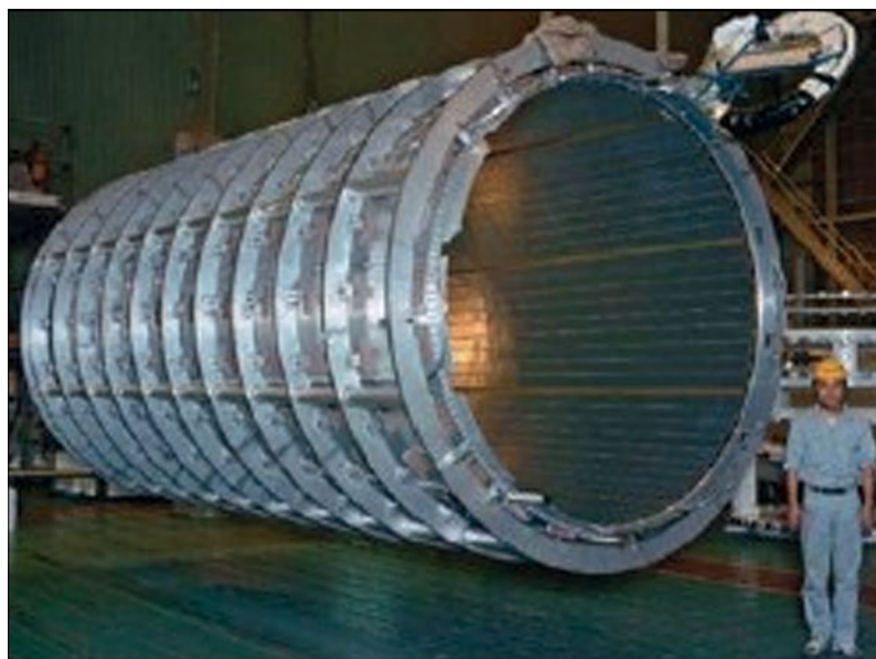
Figure 1. The central coil of the ATLAS solenoid (before being placed in its cryostat), a key component of the ATLAS interaction region at the Large Hadron Collider at CERN. It is the smallest coil in a complex superconducting magnet system containing 24 larger toroidal magnets.
