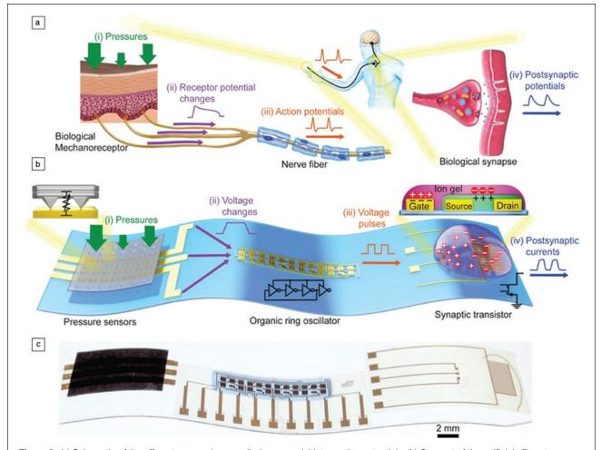
Figure 3. (a) Schematic of the afferent nerve, where applied pressure initiates action potentials. (b) Concept of the artificial afferent nerve comprising pressure sensors, a ring oscillator, and a three-terminal neuromorphic device (synaptic transistor). (c) Photograph of an artificial afferent nerve. Reprinted with permission from Reference 54. © 2018 AAAS.
