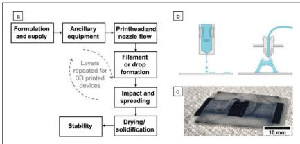
Figure 4. (a) During additive manufacturing, organic materials will undergo multiple steps, where studies will be needed to determine the effect on final functionality.6 (b) Inkjet printing (left) and fused deposition modeling (right).<sup>67</sup> Images courtesy of E. Rognin, University of Cambridge. (c) Digital photo of a 3D printed transistor channel, with the overall device 35 mm in length. Image courtesy of T. Mangoma, University of Cambridge.
