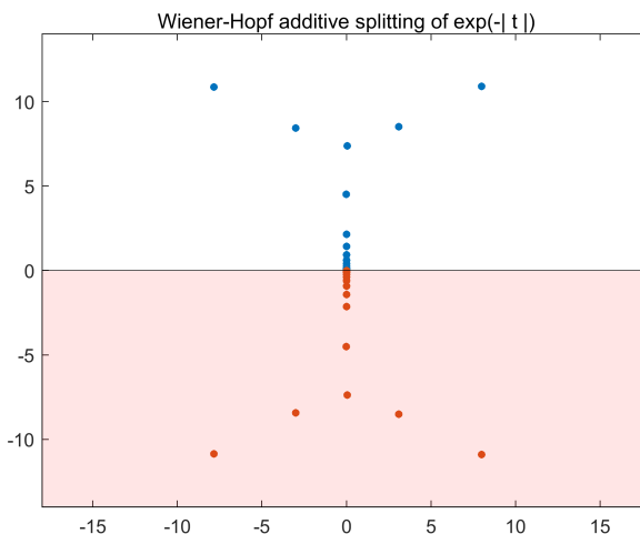
Figure 23.2. Poles of a AAA rational approximation to h(t) = e^{-|t|} for t \in \mathbb{R} . To decompose h approximately into f_+ + f_- , the contributions from the poles above and below the real axis are separated. Here there are 41 poles in each half-plane and the combination gives 10-digit accuracy.
