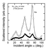
Figure 7. Incident angle dependence of Ga and In scattered intensity at the  $[11\overline{2}0]$  azimuth for  $In_{0.5}Ga_{0.5}N$  SQW. Variation of both the Ga and In signals indicates +c polarity judging from the CAICISS results on ZnO bulk given in Fig. 5. Indium atoms incorporated into an  $In_xGa_{1-x}N$  SQW were found to occupy substitutional Ga sites. [52]]
