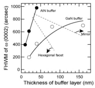
Figure 19. The FWHM value of  $\omega$  (0002) for 1  $\mu m$  HT-GaN films deposited on AlN (closed circles) and GaN (open circles) buffer layers with the thicknesses in the figure. The buffer layers were annealed for 10min under the optimum ambient. Their polarity changed as indicated by the surface morphology, and the polarity conversion occurred drastically in the case of the AlN buffer layer.
