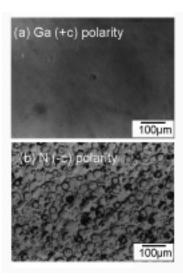
Figure 2. Optical microscope images of (a) +c GaN and (b) -c GaN films on sapphire substrates. The surface morphology of typical +c and -c GaN films are smooth and hexagonal facetted, respectively. The polarity was determined by the CAICISS method described in Sec. 2.4.
