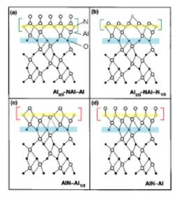
Figure 9. Models for the AlN thin films on c-plane sapphire substrates given in Ref. [58]. The color regions are added to explain the theoretical predictions. The structures in the brackets correspond to the polar structures of AlN described in Ref. [84]. (a) and (b) correspond to a +c polar surface. (c) and (d) to -c polarity.
