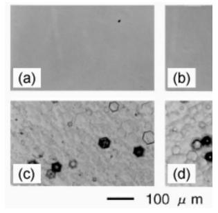
Figure 20. Influence on surface morphology of HT-GaN films of the V/III ratio in AlN buffer layers deposited at 1040 °C; V/III ratio= (a) 600, (b) 1800, (c) 6800, and (d) 13700. [127] ] A lower V/III ratio was required for the deposition of AlN buffer layer in order to obtain +c GaN film.
