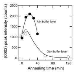
Figure 17. Variation of (0002) peak intensity of LT-GaN (open circles) and AlN (closed circles) buffer layers of 20nm thickness as a function of annealing time. The intensity was enhanced due to the crystallization of the samples induced by the annealing, and it subsequently decreased due to the layer being thinned by sublimation. This indicates that the effects of mass transportation and sublimation are smaller for AlN buffer layers.
