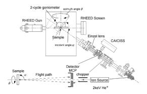
Figure 3. Schematic illustration of CAICISS apparatus with a chamber and block diagram. The incident and azimuth angles of the ion beam can be altered by moving the sample holder, which is equipped with a heater.
