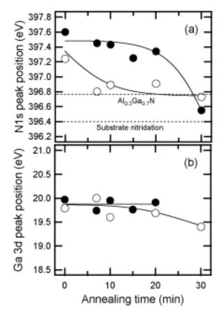
Figure 14. Dependence of (a) N1s and (b) Ga 3d peak positions for a 20-nm-thickness GaN buffer layer on  $\rm H_2$  cleaned (open circles) and nitrided (closed circles) sapphire substrates on the annealing time under the  $\rm N_2$  and  $\rm H_2$  mixed ambient. The positions were detected by XPS analysis. [after Ref. 117 ] The sample on the nitrided substrate evaporated completely, and AlGaN was formed at the interface between the sample and the non-nitrided substrate.
