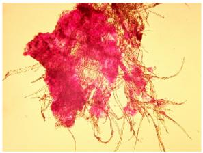
FIG. 3. Lactofuchsin stain of a paper defect. 10X
