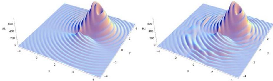
Fig.1. Absolute radial magnetic field in the x-y plane for 785nm wavelength, N.A.=1.25, objective filling factor of 1.8, and beam waist at (1.5,1.5,1.5) $\mu$ m: (left) theoretical field; (right) Exact Partial Wave reconstruction for just the first 30 terms.
