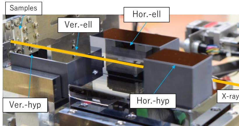
**Figure 2.** Photograph of the developed imaging mirrors.
