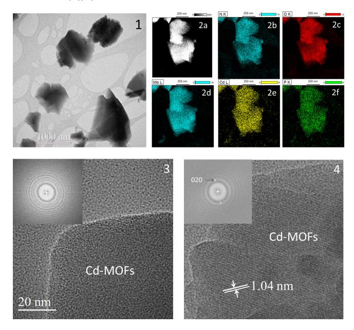
Figure 1. Bright-field TEM image of Cd-MOFs crystals showing sample morphology.
