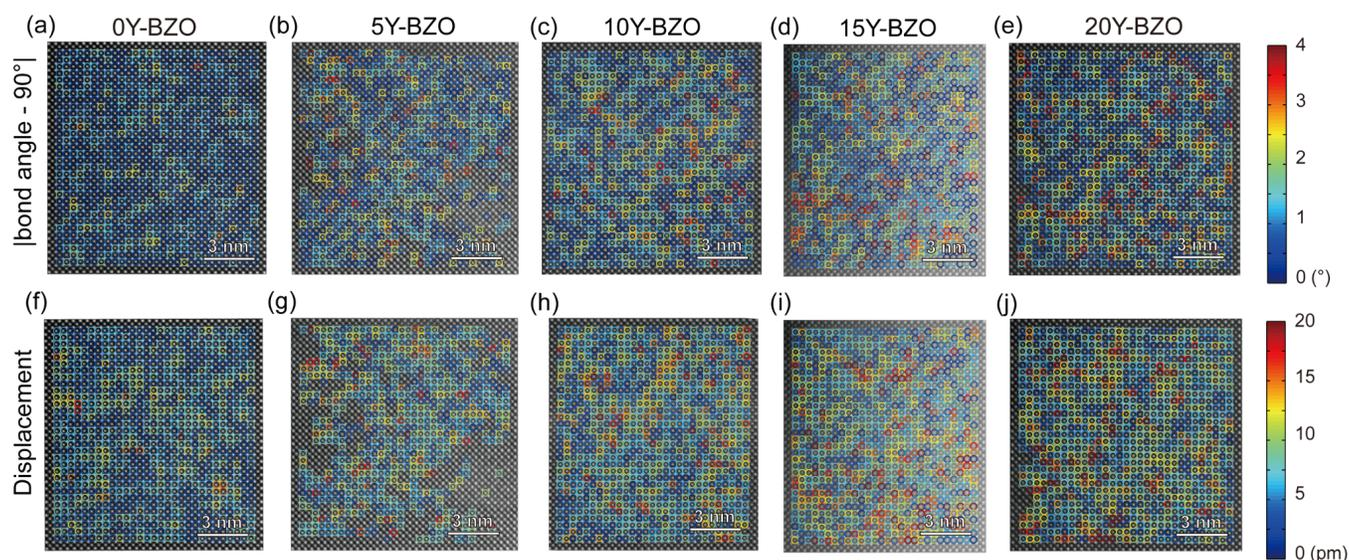
**Figure 1.** Aberration-corrected ADF-STEM images overlaid with measurements for (a-e) B-site bond angle deviation for 0Y-BZO - 20Y-BZO and (f-j) B-site atomic displacement for 0Y-BZO - 20Y-BZO.
