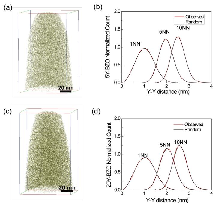
**Figure 2.** APT reconstructed volumes showing homogeneous distribution of Y dopants and distribution of 1<sup>st</sup>, 5<sup>th</sup>, and 10<sup>th</sup> Y-Y nearest neighbor for (a-b) 5Y-BZO and (c-d) 20Y-BZO.
