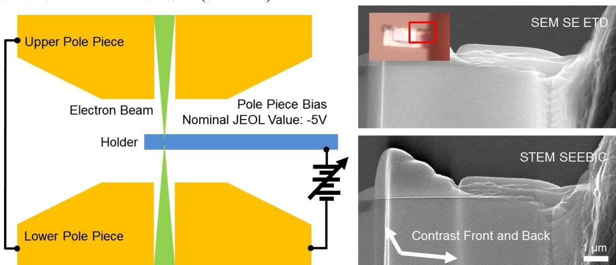
**Figure 1.** (left) Pole piece and bias voltage geometry. FIB-prepared lamella (optical image inset, ROI selected) imaged with an Everhart-Thornley detector (ETD) in an SEM (right top), and with SEEBIC in a STEM (right bottom).
