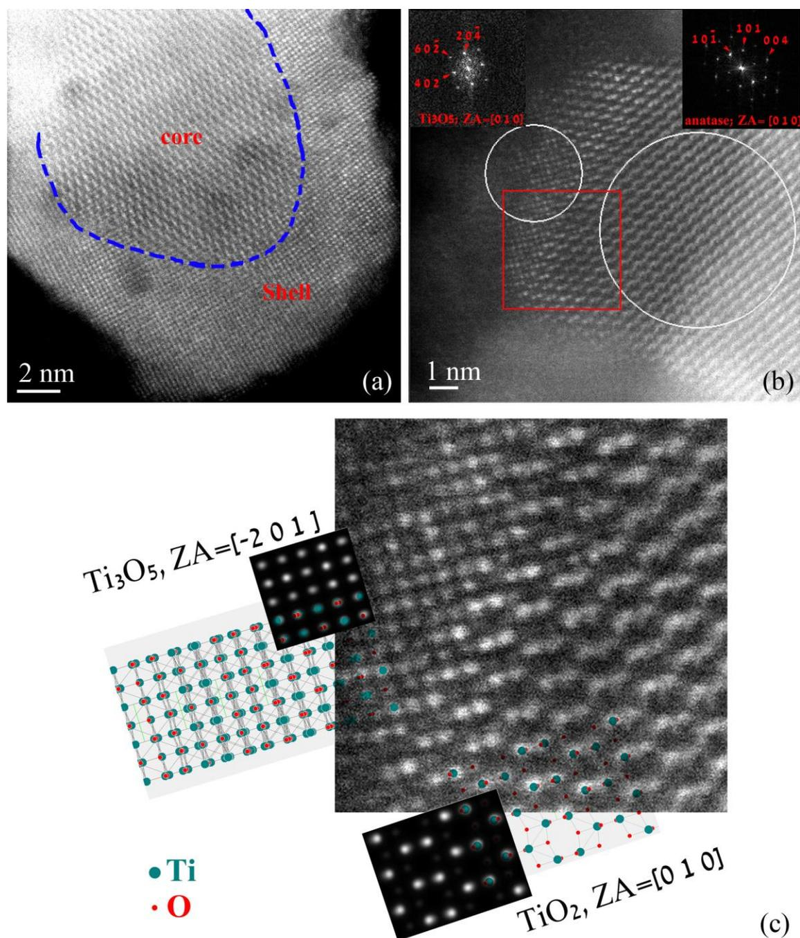
**Figure 1.** (a) TEM micrograph of  $\text{Ti}_3\text{O}_5$  at low magnification. (b) SAED taken from the green boxed area shows presence of  $(203)$ ,  $(402)$  and  $(-602)$  planes of monoclinic  $\text{Ti}_3\text{O}_5$  and the corresponding intensity profile of anatase (inset).
