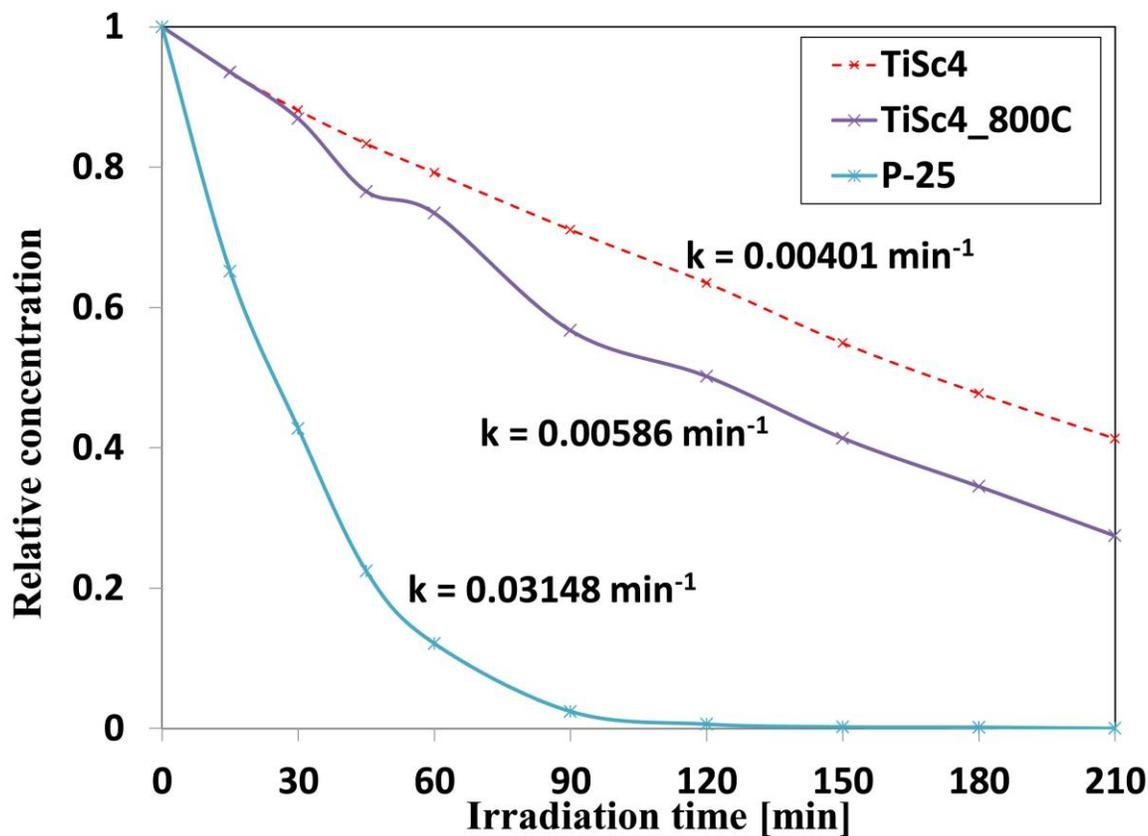
**Figure 2.** Decomposition of methylparation under UV light on TiSc4 and annealed TiSc4-800 samples, and standard P25.
