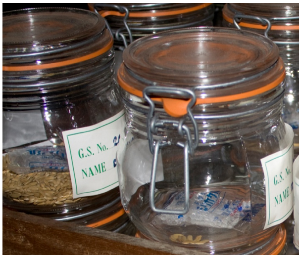
Fig. 1. Genebank seed storage in glass jars with rubber sealing, showing relatively large ratios of enclosed oxygen to the number of stored seeds.
