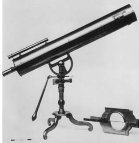
Figure 1. Gregorian reflector 1900-136, by Short, with object-glass micrometer (Courtesy: Science Museum, Science and Society Picture Library).
