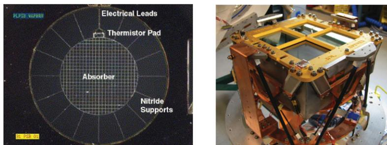
**Figure 4.** At left, a polarization sensitive bolometer, as employed in the 2003 flight of Boomerang, Bicep, QUaD and the *Planck* HFI instrument (Jones *et al.* 2003). At right, one of *Spider*'s six large format arrays of 512 antenna-coupled detectors (Bonetti *et al.* 2012).
