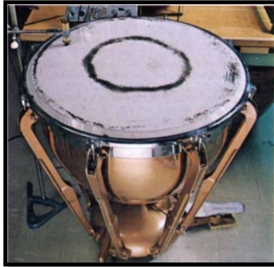
Fig. 3. Standing wave pattern on a kettledrum head. One of many possible standing wave patterns on a kettledrum head, made visible by dark powder sprinkled on the drumhead. As the head is set into oscillation at a single frequency by a mechanical oscillator at the upper left of the photograph, the powder collects at the nodes. By the same way, due to the oscillation of the solar system wave function the dust grains and gas of the solar system protoplanetary disk were grouped in certain orbits.
