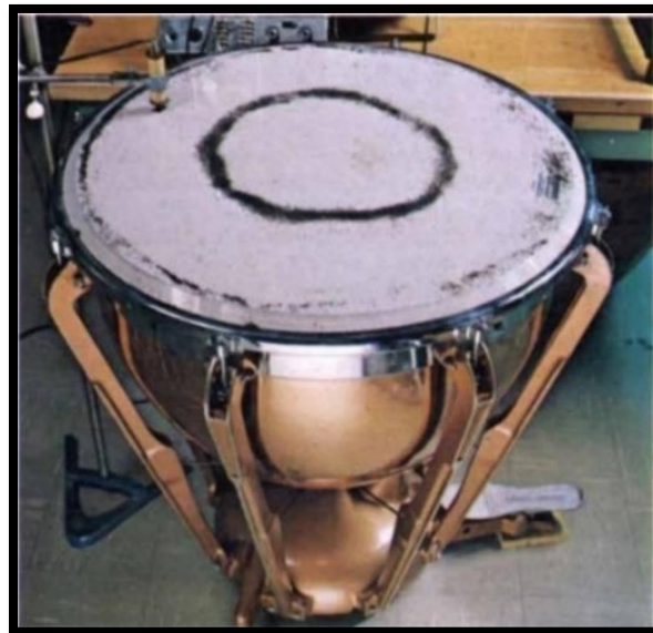
Fig. 3. Standing wave pattern on a kettledrum head. One of many possible standing wave patterns on a kettledrum head, made visible by dark powder sprinkled on the drumhead. As the head is set into oscillation at a single frequency by a mechanical oscillator at the upper left of the photograph, the powder collects at the nodes. By the same way, due to the oscillation of the solar system wave function the dust grains and gas of the solar system protoplanetary disk were collected in certain orbits.
