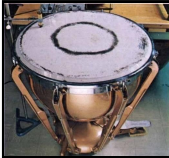
Fig. 3. Standing wave pattern on a kettledrum head. One of many possible standing wave patterns on a kettledrum head, made visible by dark powder sprinkled on the drumhead. As the head is set into oscillation at a single frequency by a mechanical oscillator at the upper left of the photograph, the powder collects at the nodes. Similarly, due to the oscillation of the solar system wave function the dust grains and gas of the solar system protoplanetary disk were collected in certain orbits.
