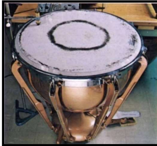
Fig. 3. Standing wave pattern on a kettledrum head. One of many possible standing wave patterns on a kettledrum head, made visible by dark powder sprinkled on the drumhead. As the head is set into oscillation at a single frequency by a mechanical oscillator at the upper left of the photograph, the powder collects at the nodes. Similarly, due to the oscillation of the SSWP the dust grains and gas of the solar system protoplanetary disk were collected in certain orbits.
