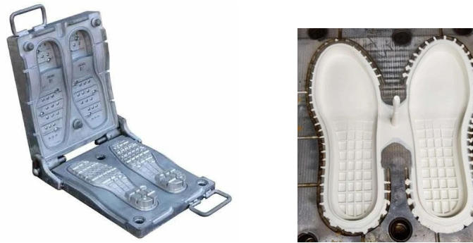
Figure 1. Molds used for manufacturing a pair of rubber soles.
