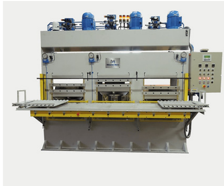
Figure 3. Vulcanization machines with one or more presses, each composed by several slots for positioning the molds.
