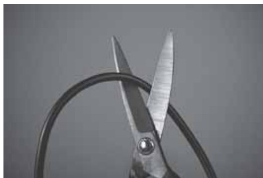
Scissors gently scraping the plastic off insulated wire
