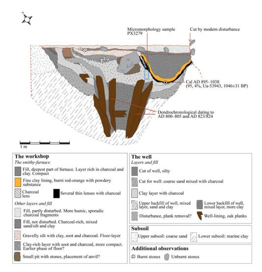
Figure 6. Section through the workshop and underlying well.
