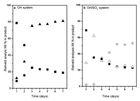
FIG. 2. Rietveld analysis for kaolinite aged in 5 M NaOH (a) and 5 M NaOH/SO<sub>4</sub> (b) at 70°C for 7 days. Mineral wt.% are shown for kaolinite (squares), sodalite (triangles), cancrinite (circles) and vishnevite (stars). Muscovite impurity in the starting material is not shown.
