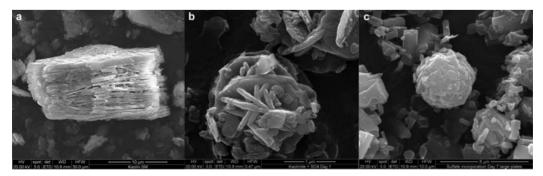
FIG. 3. SEM images for kaolinite (a) and the alkaline alteration product formed during the ageing of kaolinite in  $5 \text{ M NaOH} + \text{SO}_4 (4 \text{ M})$  at 70°C for (b) 2 days and (c) 7 days.
