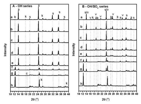
FIG. 1. X-ray diffraction (XRD) patterns of kaolinite aged in 5 M NaOH (A) and 5 M NaOH/SO<sub>4</sub> (B) at 70°C for (a) 7 days, (b) 6 days, (c) 5 days, (d) 4 days, (e) 3 days, (f) 2 days and (g) 1 day. The XRD pattern of the kaolinite starting material is shown in (h). Minerals are annotated as s (sodalite), k (kaolinite), v (vishnevite) and c (cancrinite).
