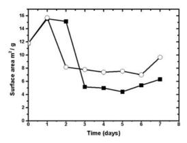
FIG. 4. Changes in mineral surface area during the reaction of kaolinite in 5 M NaOH (circles) and NaOH/SO<sub>4</sub> (squares) at  $70^{\circ}$ C for 7 days.
