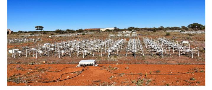
Figure 3. The CRAM as installed at the centre of the southern hexagon array of the MWA Phase II configuration, looking west. In the lower centre of the image is the second-stage beamformer, first-stage beamformers are visible on the left and right of the image.
