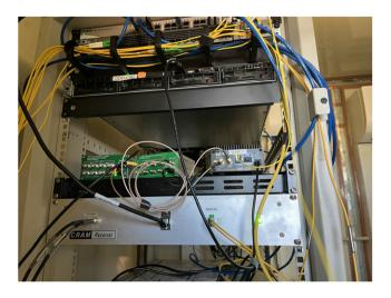
Figure 8. The CRAM receiver unit placed inside the T-hut along with the MWA clock system.
