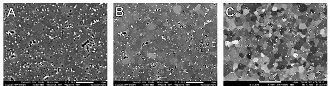
**Figure 1.** BSE Micrographs of LiAlO<sub>2</sub> ceramic specimens under low vacuum conditions. (A) 15kV with C coating; (B) 5kV with C coating; and (C) 5kV with no coating.
