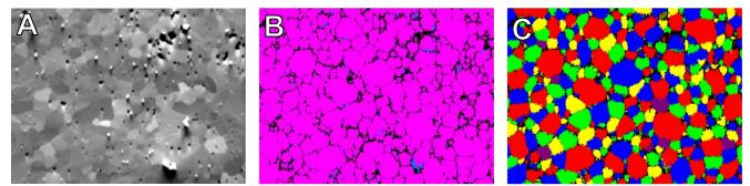
**Figure 2.** EBSD micrographs of LiAlO<sub>2</sub>: (A) forscatter , (B) phase map (magenta = LiAlO<sub>2</sub>, blue =  $LiAl_5O_8$ ), and (C) grain size.
