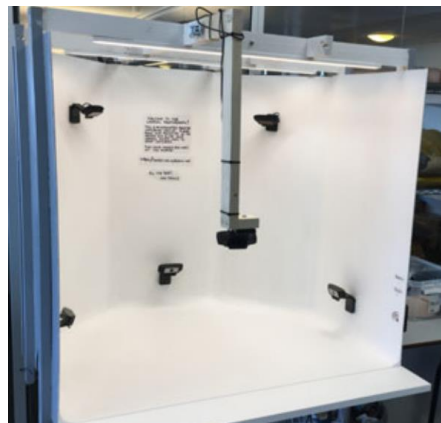
Figure 1. Updated version of Protoboosth showing the seven camera positions (one camera at top dead centre of the booth) (Erichsen et al., 2021)
