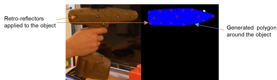
Figure 3. Reflectors and ICP on drill prototype
