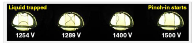
Figure 7. First demonstration of dielectrophoretic behavior in a cryogenic liquid: electrostatic field has been used to levitate a column of liquid D 2 and form a droplet of the desired volume (taken from Ref. [77]).
