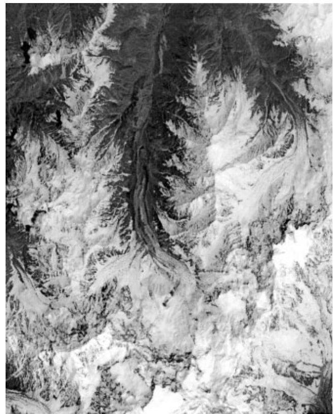
Fig. 4. SPOT 3 spectral band 3 image of the Raikot basin. Differential illumination is present at a variety of scales. High-frequency reflectance variation is clearly visible and highlights the terrain. The terminus of Raikot Glacier can be seen.
