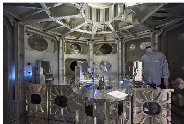
Figure 23. Working inside P3. The interior of the P3 experimental chamber is treated as a cleanliness class ISO 5 cleanroom, whereas the experimental hall E3 is an ISO 7 cleanroom.
