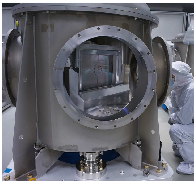
Figure 10. Mounted HAPLS BT mirror installed in its vacuum chamber and both, chamber and breadboard legs/feet bolted onto the aluminium chamber base plate in ISO 5 class cleanroom.
