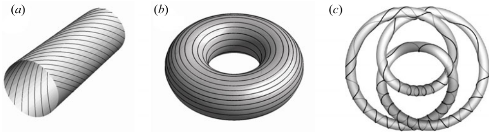
Figure 2. Isosurfaces of the exact VSF: (a) vortex column in the integrable ABC flow, (b) vortex ring and (c) knotted vortex tube. Some vortex lines are integrated from points on the isosurfaces.
