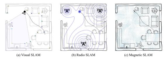
Figure 1. Illustration of the different SLAM modalities used throughout this paper. (a) Visual SLAM uses a sparse map representation of distinctive corner points observed as projections onto the camera frustum, (b) radio SLAM either uses a sparse map of the radio emitter locations or models the RSSI anomalies as a dense field, and (c) magnetic SLAM leverages anomalies in the local magnetic vector field.
