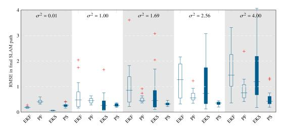
Figure 6. Robustness to feature point initialization in visual SLAM. Simulation study with initial feature locations perturbed with Gaussian noise (variance  $\sigma^2$ ). Box plots of RMSE in the final estimated SLAM path. Forward filtering methods drawn with outlines, smoothing methods in solid colors. The EKF/EKS perform well under negligible perturbation, the particle filter (PF) and smoother (PS) perform well under large uncertainty.
