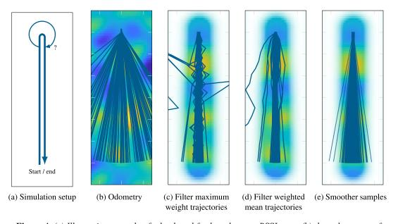
Figure 4. (a) Illustrative example of a back and forth path on an RSSI map; (b) the only source of uncertainty in the odometry is the turn angle at the farthest most point, which leads to spread; (c, d) Particle filtering SLAM reduces the spread, but does not backtrack the smooth odometry information; and (e) Our particle smoothing solution gives a tighter estimate and backtracks the smoothness along the sample paths.
