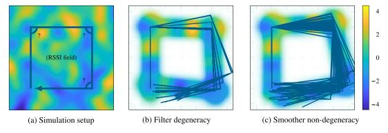
**Figure 3.** Highlight of the non-degeneracy of the particle smoothing approach with (a) the simulation setup, and simulation results for radio SLAM with (b) filtering samples showing that the filter is degenerate and (c) nondegenerate samples of the smoother.
