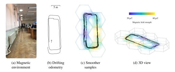
**Figure 7.** Empirical proof-of-concept magnetic indoor SLAM. Panel (a) shows a view through the mobile phone camera, (b) the drifting odometry, (c) samples of the smoothing distribution, and (d) a 3D view of these results. The color scaling visualizes the field strength of a learned magnetic map.
