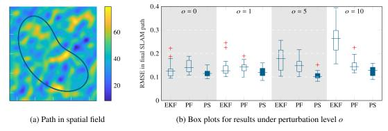
Figure 5. Robustness study with magnetometer perturbed with a constant bias o. Left: Setup showing the ground-truth path and one realization of the magnetic field map. Right: Box plots of RMSE in the final estimated SLAM path. Particle and extended Kalman filtering methods drawn with outlines, particle smoothing method in solid colors. The EKF performs well under negligible calibration errors, the particle filter (PF) and smoother (PS) perform well under large calibration errors.
