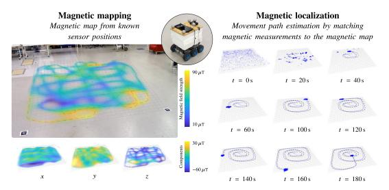
Figure 2. Left: A magnetic anomaly map mapped by a robot (smartphone for scale) equipped with a three-axis magnetometer. Map opacity follows the marginal variance (uncertainty), and mapping (training) paths shown by dashed lines. Right: Localization by map matching. Current estimate is characterized by a particle cloud, the dashed line shows the ground-truth, and the solid line the weighted mean path.
