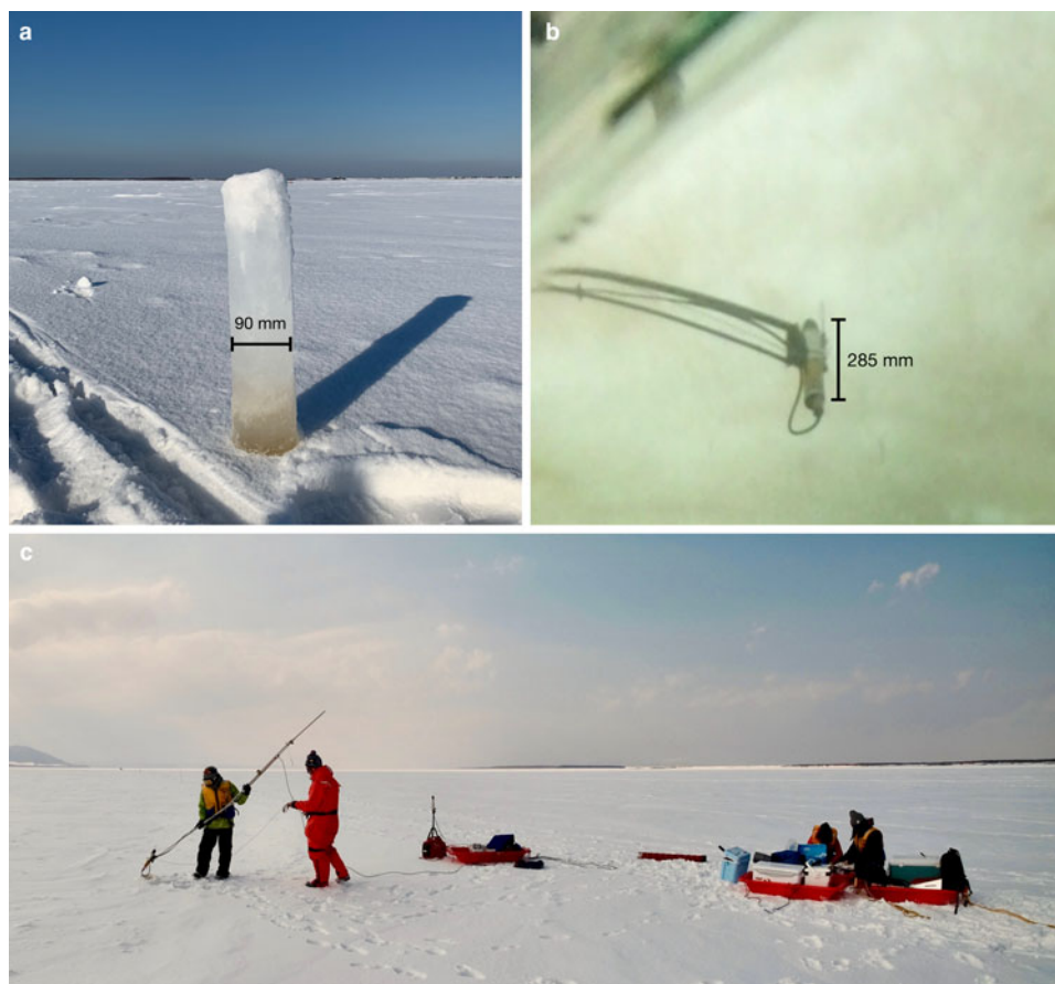
Fig. 2. Integrated physico-biogeochemical observations at Saroma-ko Lagoon. (a) A typical 90 mm diameter sea-ice core from Saroma-ko Lagoon. (b) Under-ice irradiance sensor in operation. This sensor was measuring the light transmitted through snow, sea ice and absorbed by sea-ice algae. (c) Deployment of the irradiance sensor through the borehole (as in (b)) with concomitant measurement of a temperature profile by other team members. Pictures (b) and (c) were taken from Nomura and others (2020), with permission from the Bulletin of Glaciological Research, the Japanese Society of Snow and Ice.
