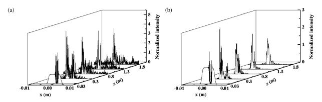
Figure 7. The propagation of a narrowband beam (a) and a broadband beam (b) when the defect is not in the centre,  $x_0 = 0.001$  m; the other parameters are the same as in Figure 6.
