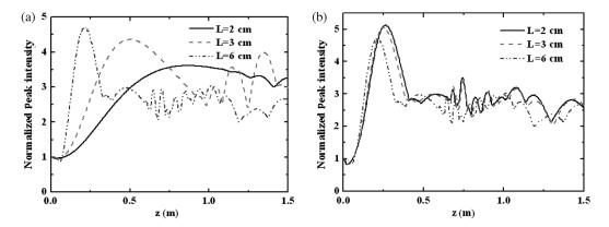
Figure 3. (Colour online) Evolution of the normalized peak intensity of a broadband super-Gaussian beam passing through different thicknesses of nonlinear medium along the propagation direction. (a) The incident intensity is fixed,  $I_0 = 12 \text{ GW/cm}^2$ . (b) The B integral is fixed,  $I_0 = 36 \text{ GW/cm}^2$ when L = 2 cm;  $I_0 = 24$  GW/cm<sup>2</sup> when L = 3 cm;  $I_0 = 12$  GW/cm<sup>2</sup> when L = 6 cm. N = 4,  $w_0 = 3$  mm, and  $\Delta \lambda = 40$  nm.
