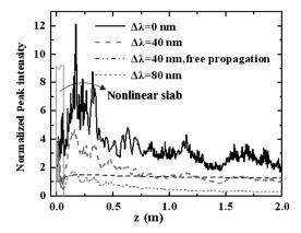
Figure 5. (Colour online) Evolution of the normalized peak intensity of a super-Gaussian beam for different bandwidths, considering the medium's front surface to have a defect. The defect size  $a = 100 \mu m$ , A = 1,  $x_0 = 0$ ;  $n_0(\lambda_0) = 1.812$ ,  $n_2(\lambda_0) = 2.28 \times 10^{-6}$  cm<sup>2</sup>/GW, L = 6 cm,  $I_0 = 12 \text{ GW/cm}^2$ , N = 4, and  $w_0 = 3 \text{ mm}$ .
