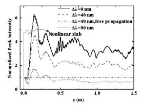
**Figure 2.** (Colour online) The normalized peak intensity of a super-Gaussian beam against the propagation distance for different bandwidths.  $n_0(\lambda_0) = 1.812$ ,  $n_2(\lambda_0) = 2.28 \times 10^{-6}$  cm<sup>2</sup>/GW, L = 6 cm, the super-Gaussian beam  $I_0 = 12$  GW/cm<sup>2</sup>, N = 4, and  $w_0 = 3$  mm.
