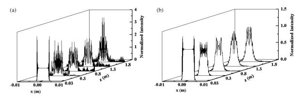
Figure 4. Intensity distribution of a narrowband beam,  $\Delta \lambda = 0$  nm (a) and a broadband beam,  $\Delta \lambda = 40$  nm (b) at different distances.  $n_0(\lambda_0) = 1.812$ ,  $n_2(\lambda_0) = 2.28 \times 10^{-6} \text{ cm}^2/\text{GW}, L = 6 \text{ cm}, I_0 = 12 \text{ GW/cm}^2, N = 20, \text{ and } w_0 = 3 \text{ mm}.$
