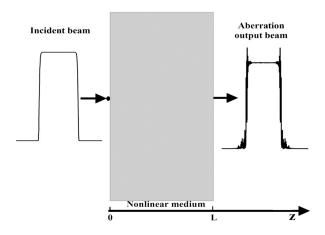
Figure 1. (Colour online) Schematic illustration of a super-Gaussian beam passing through a nonlinear medium.
