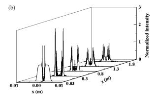
Figure 6. The propagation of a narrowband beam,  $\Delta \lambda = 0$  nm (a) and a broadband beam,  $\Delta \lambda = 40$  nm (b) through a nonlinear medium whose front surface contains a defect. Here, the parameters are the same as in Figure 5.
