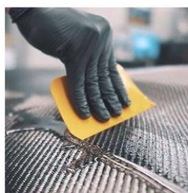
(b) Carbon Fibre Layup
