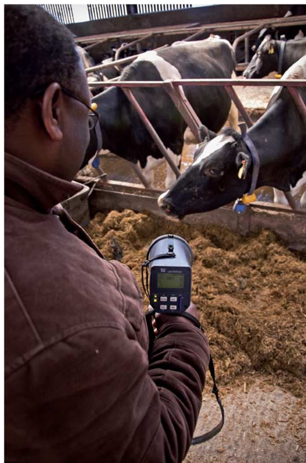
Figure 1 A demonstration on the use of the Laser Methane Detector in livestock. Picture: A. Ross.
